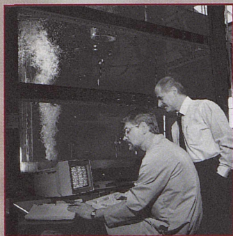
Achilles Vassilicos (standing) with Ron Woodrow of the U.S. Steel Technical Center staff in the "flow lab," analyzing results from a physical model of gas stirring in a steel ladle.
