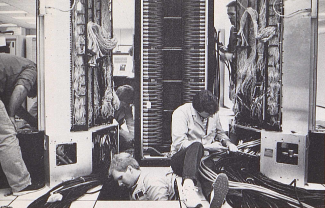
The Cray installation team at work on "the Y." Laced piping in the processor carries the liquid that cools the Y's circuitry.
