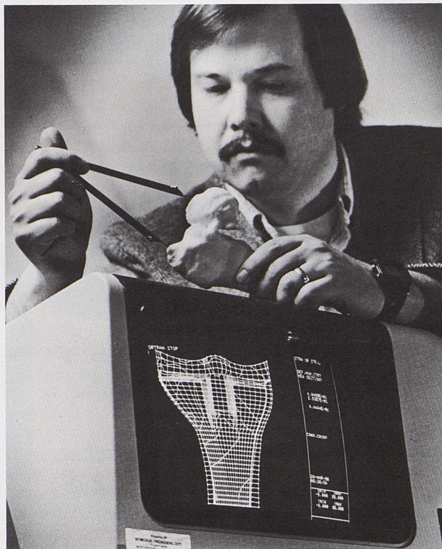
Richard Hart stands over a monitor which displays a two-dimensional finite element model of the human tibia with the lower portion of a prosthetic knee replacement. The closely packed stress contours indicate where the prosthetic material could fail.
