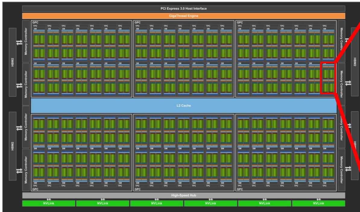
Volta GV100 GPU with 85 Streaming Multiprocessor (SM) units
