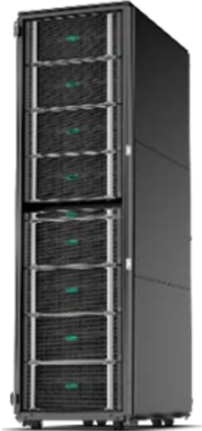
HPE Superdome Flex HPC Server
